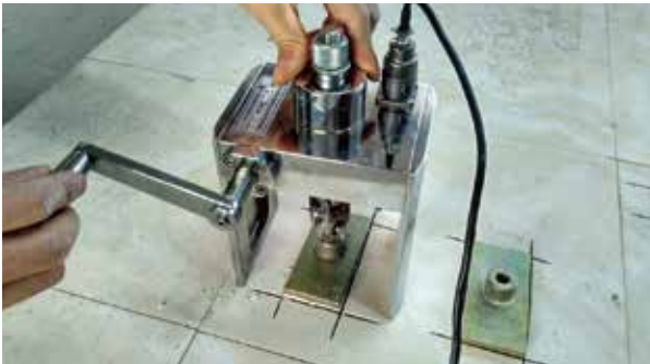
Ceramic tile drawing force test
